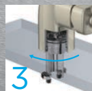
Twist faucet into place Tournez robinet en place
